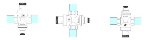
The pressure reducers MINIBRASS don't get the effects, in their functioning, of gravity force; therefore they can be installed in the plant in any position:
